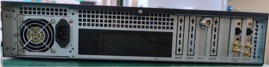
Front panel power switch, rear panel with battery connector, main antenna connector (N type), GSM frequency sweep antenna connector (SMA-K), LTE frequency sweep antenna connector (SMA-K), network port connector (RJ45)
